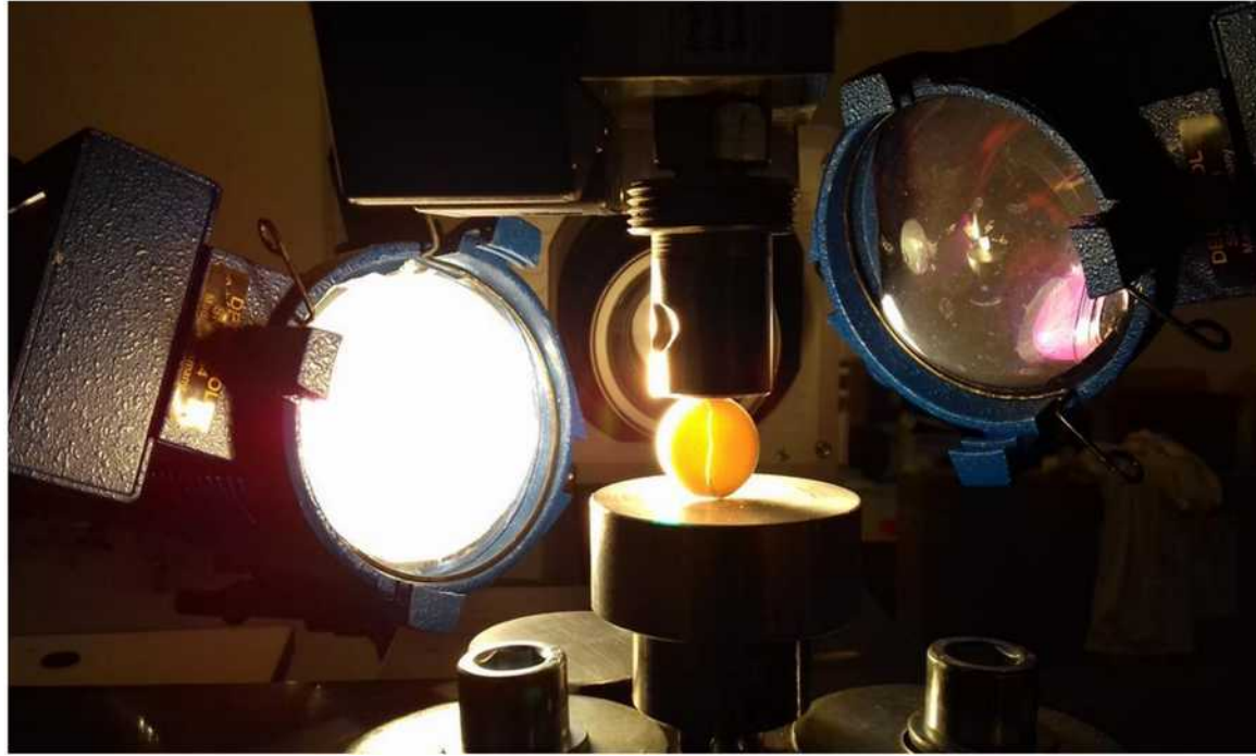
Brazilian test on a pharmaceutical compress (diameter = 11mm)
