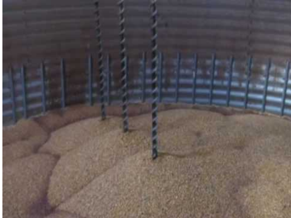
Grain silo – 3-rotating dryer
